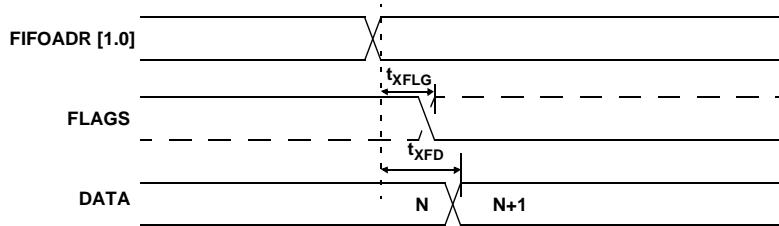
**Figure 9-12. Slave FIFO Address to Flags/Data Timing Diagram**
