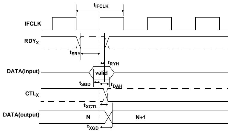
**Figure 9-4. GPIF Synchronous Signals Timing Diagram**
