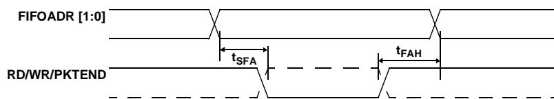
**Figure 9-14. Slave FIFO Asynchronous Address Timing Diagram**
