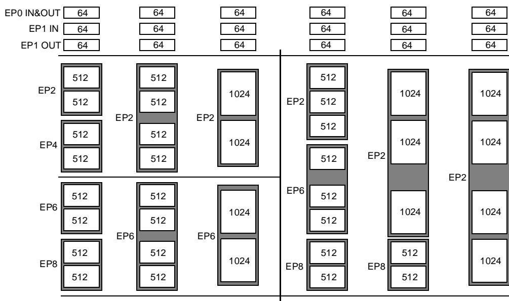
**Figure 3-4. Endpoint Configuration**
