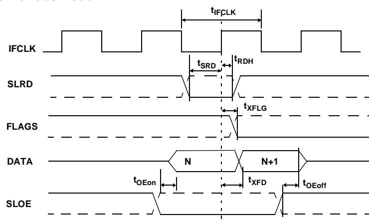
**Figure 9-5. Slave FIFO Synchronous Read Timing Diagram**
