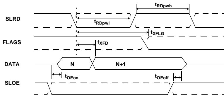
**Figure 9-6. Slave FIFO Asynchronous Read Timing Diagram**
