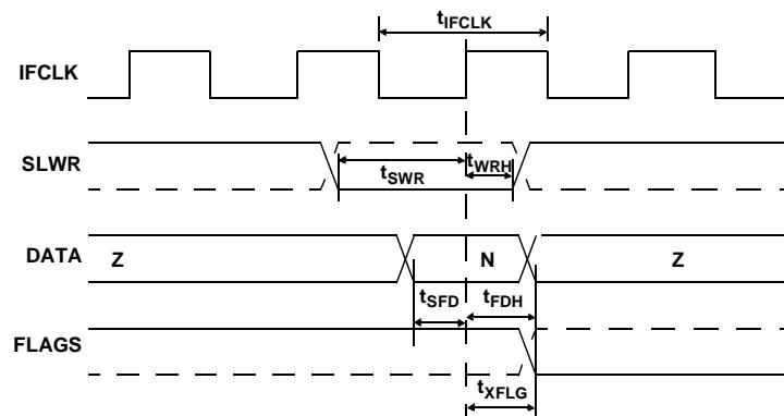
**Figure 9-7. Slave FIFO Synchronous Write Timing Diagram**
