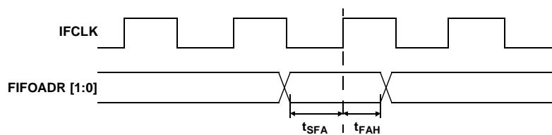
**Figure 9-13. Slave FIFO Synchronous Address Timing Diagram**
