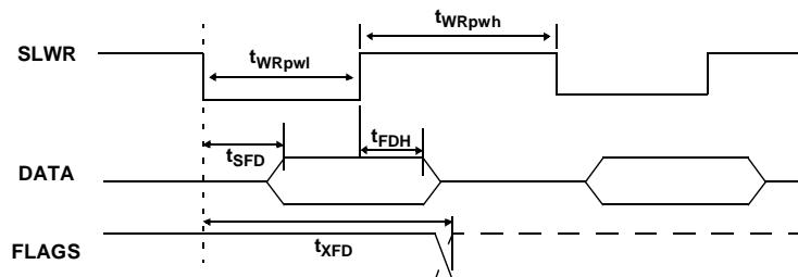
**Figure 9-8. Slave FIFO Asynchronous Write Timing Diagram**
