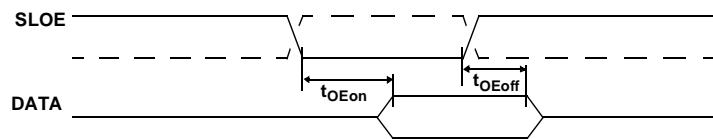
**Figure 9-11. Slave FIFO Output Enable Timing Diagram**
